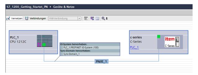
Figure 5-2: IO controller assignment under SIEMENS S7
