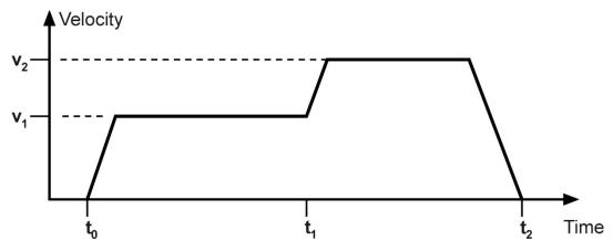
Figure 11-1: Uninterrupted sequence of motion tasks
