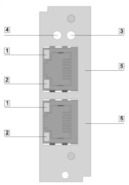
Figure 3-2: Connection and display elements of the PROFINET module
