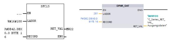
Figure 13-3 STEP7 Block with initial address of the A-area
