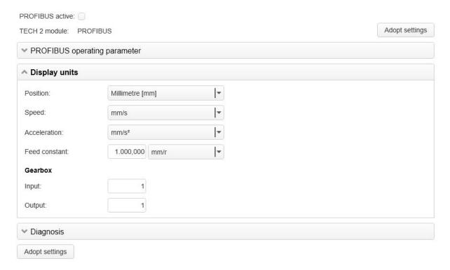
Figure 7-1: Setting of physical units for PROFIBUS
