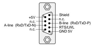
Figure 3-1: PROFIBUS connector for item C-Series
