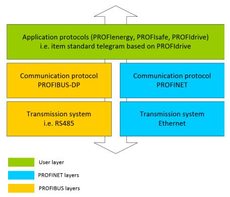
Figure 4-1: Comparison of PROFIBUS and PROFINET
