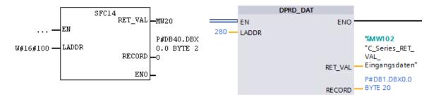
Figure 13-1 STEP7 Block with initial address of the E-area
