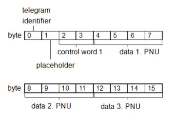
Figure 6-1: Example of the item C-Series telegram format
