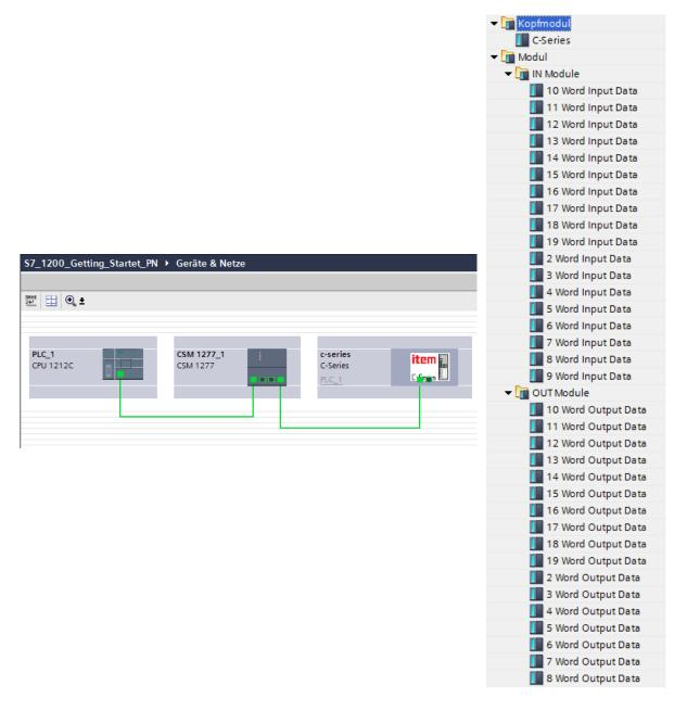
Figure 5-3: Hardware configuration under SIEMENS S7
