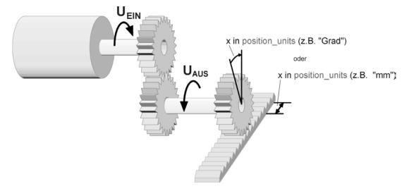
Figure 7-2: Gear ratio
