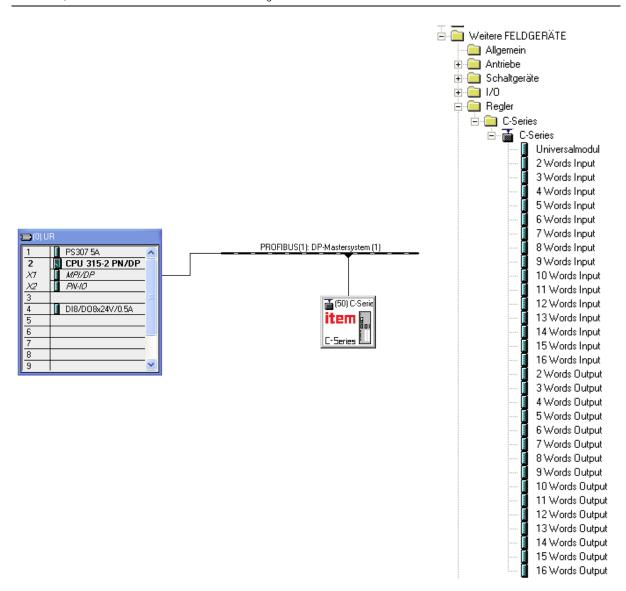
Figure 5-1: Hardware configuration under SIEMENS S7
