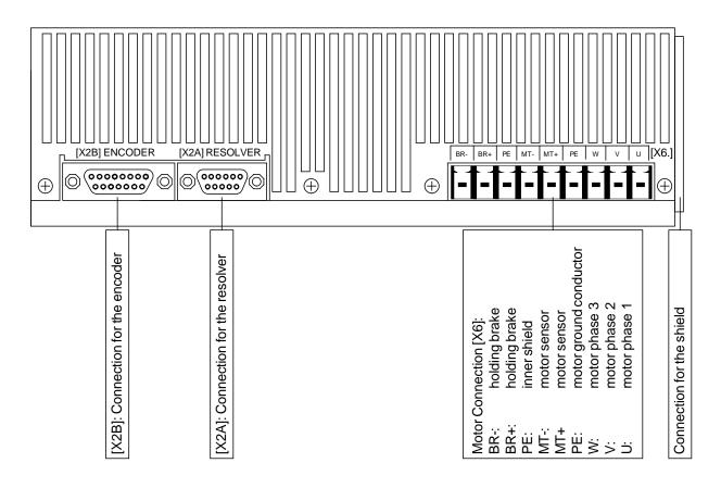
Figure 3: item Servo Positioning Controller C 3-10: Bottom view
