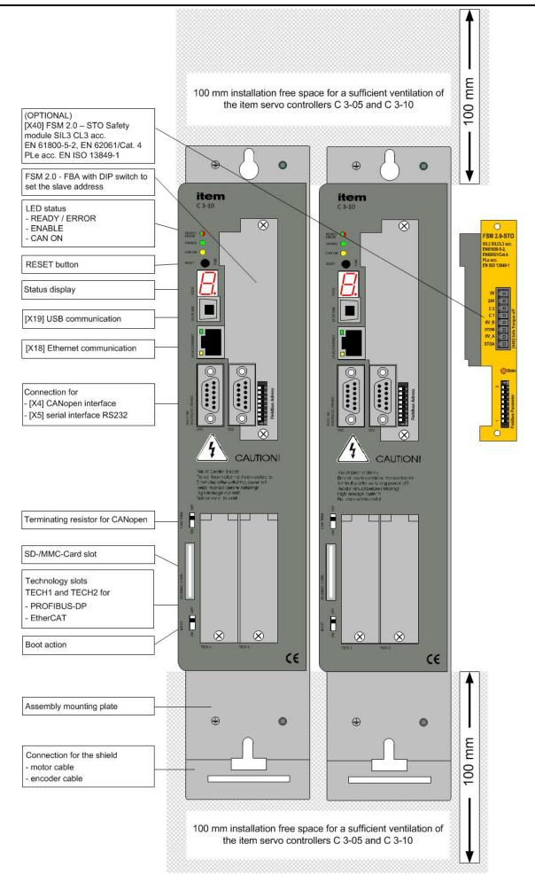
Figure 1: item Servo Positioning Controller C 3-10: Front view and Installation space
