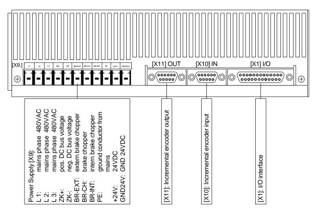
Figure 2: item Servo Positioning Controller C 3-10: Top view
