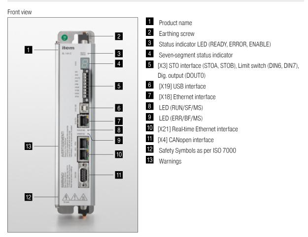
Figure 2: Front view of a BL 1-04 /C
