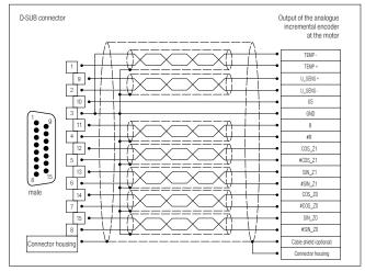
Figure 25: Pin assignment: analogue incremental encoders [X2B]
