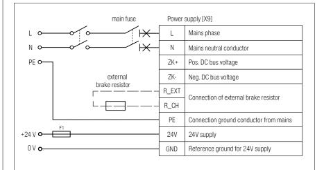
Figure 20: Connection of a BL 1-04 /C to the power supply [X9]
