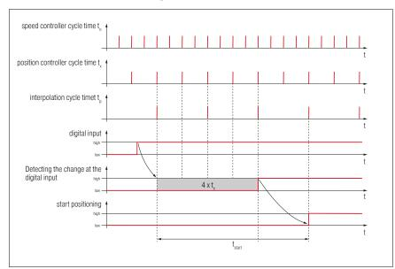
Figure 15: Filter time mechanism in the case of digital inputs
