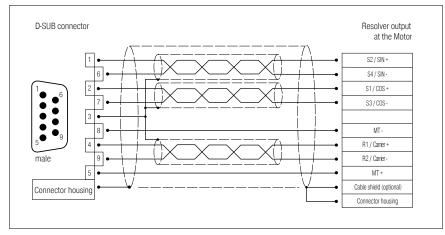
Abbildung 24: Pin assignment: resolver connector [X2A]
