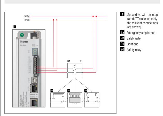
Figure 6: Connection of the integrated STO function (single-phase servo drive)
