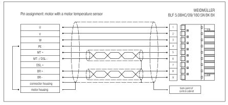
Figure 22: Pin assignment: motor connector (motor temperature sensor) [X6]
