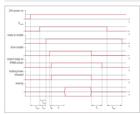
Figure 17: Time diagram of the servo drive
