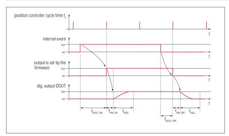
Figure 16: Filter time mechanism in the case of digital outputs
