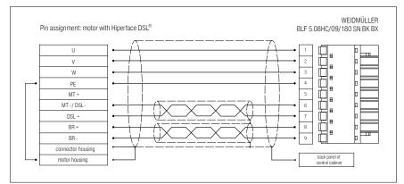
Figure 23: Pin assignment: motor connector (HIPERFACE DSL®) [X6]
