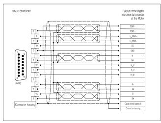
Figure 27: Pin assignment: digital incremental encoder (RS422) [X2B]
