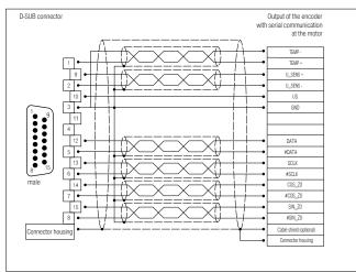
Figure 26: Pin assignment: incremental encoder with a serial interface [X2B]
