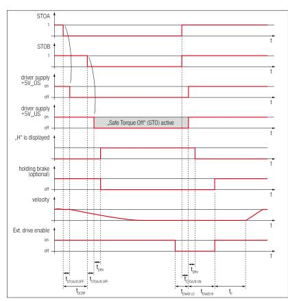
Figure 18: Time response of the activation of the STO safety function with a restart
