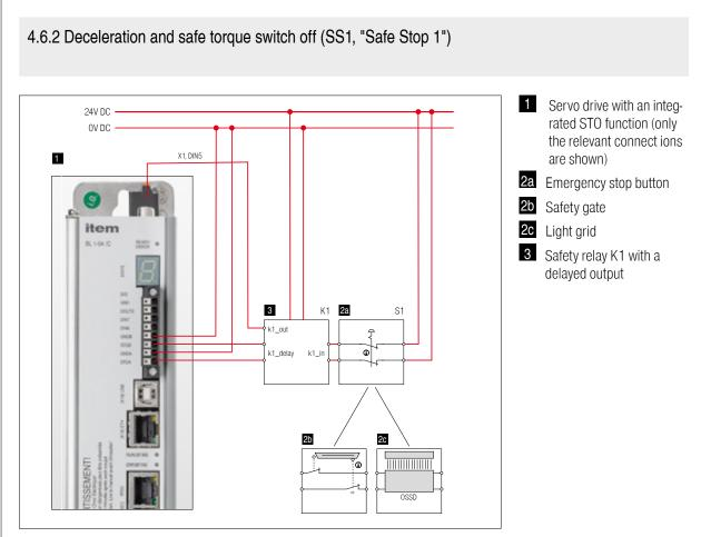
Figure 7: Circuit example "Deceleration and safe torque switch-off" (SS1, "Safe Stop 1") (single-phase servo drive)
